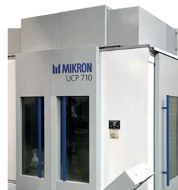
5-axis portal milling machine from Mikron for manufacturing precision parts
