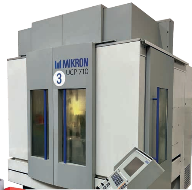
5-axis portal milling machine from Mikron for manufacturing precision parts
